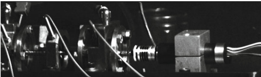
Fig. 19 Test rig shot at coupling contraction (100 Hz)
