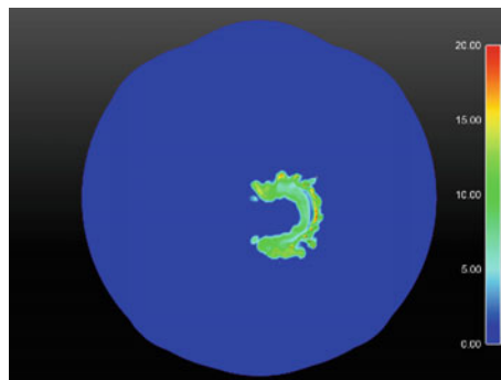
Fig. 10 Calculated overall equivalence ratios for the single injection event in a 2D plane 2 mm above the TDC position of the piston at -20^\circ CA
