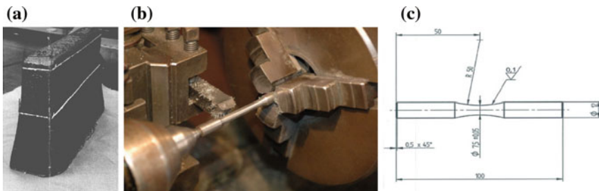
Fig. 3.1 Production of standardized specimens for rotating bending fatigue tests (ISO 1143): a metallic block from sand casting; b tool machining; c “dog-bone” shape
