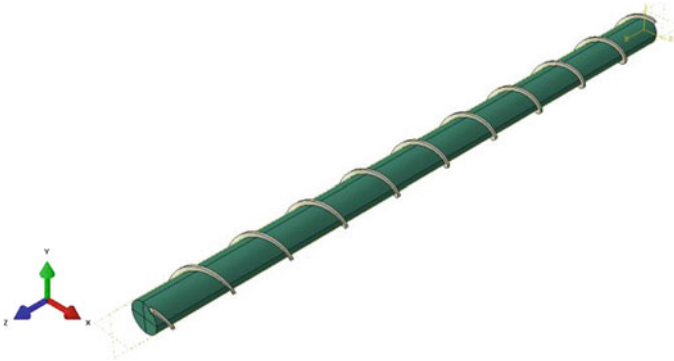
Fig. 19.3 Circular rebar with helical wrap
