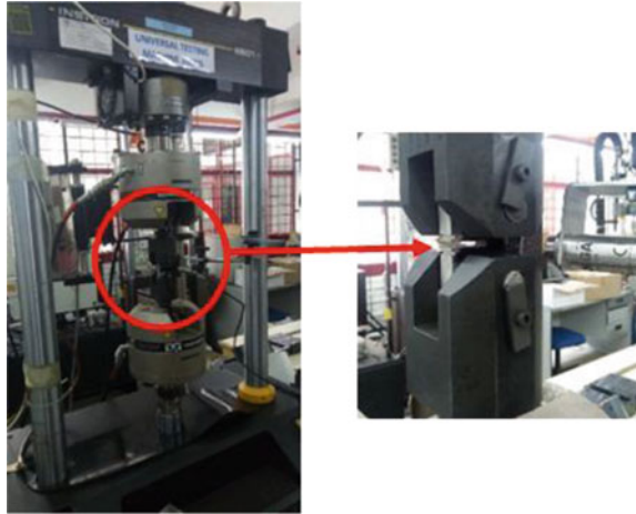
Fig. 28.2 The setup of the IR sensor and the specimen
