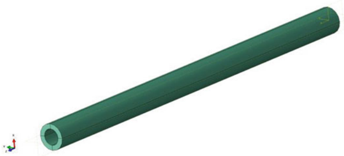
Fig. 19.4 Bar with ring cross-section
