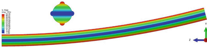
Fig. 19.9 Map of the Huber-Misses stresses expressed in megapascals for a bar with a circular cross-section with protrusions bent by 1.5°—bar material was CR144 resin reinforced (80%) with glass fiber (deformation scale \times 10 )
