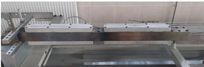
Fig. 20.1 Pultrusion die with the heating sources mounted
