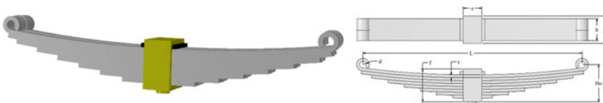
Fig. 11.5 Geometry of single-stage UIC trapezoidal leaf spring: Left—Tridimensional model; Right—Technical drawing
