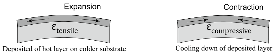
Fig. 14.2 Schematic representation highlighting basic mechanisms of residual stress and residual strain evolution throughout AM process. Adapted from [15]
