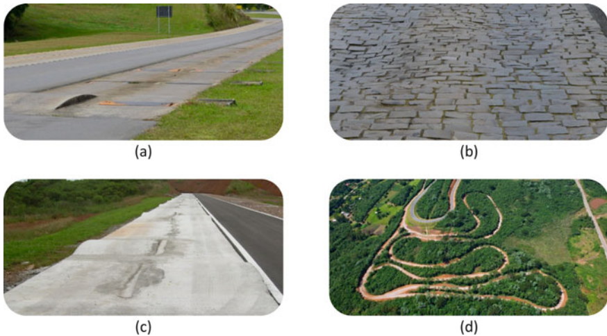
Fig. 2.2 Special test tracks: potholes (a), Belgian stones (b), body twist (c), and off-road (d)
