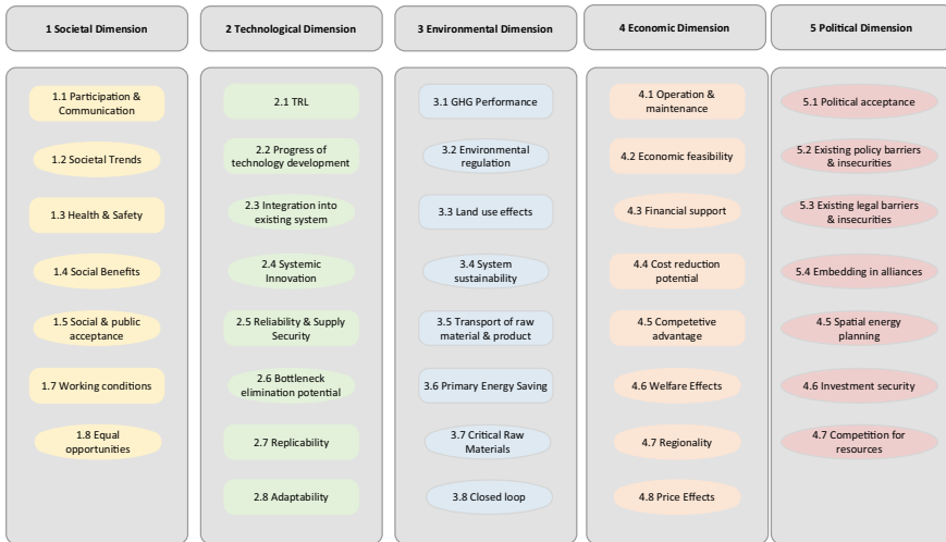
Fig. 22.3 Set of qualitative indicators for a multi-dimensional sustainability assessment of Power-to-Product Technology (source Friedl et al. [77])
