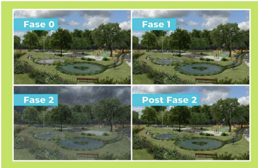
Fig. 15.3 Explanatory render of a GBI co-designed in Prato: Phase 0: dry period, part of the wetland is dry and part is wet, the swale is dry; Phase 1: during low-intensity rain events, the swale and all the wetland is wet; Phase 2: during heavy rainfall, all the NBS elements, swale and wetland, are occupied by water at full lamination capacity; Post Phase 2: the park is lived in safety
