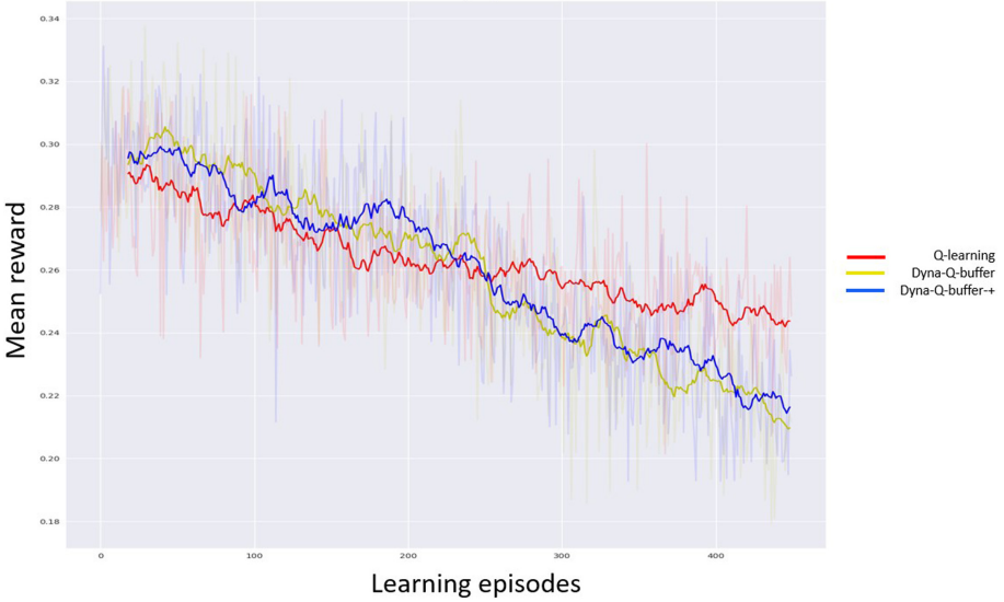
Fig. 4. Average reward over learning episodes in tandem queue environment with larger scale
