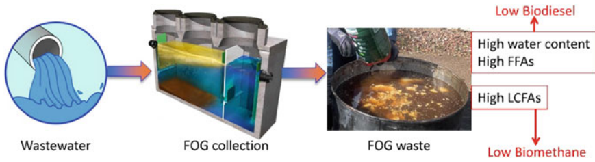
Fig. 10.1 Challenges associated to fats, oils and grease (FOG) for bioenergy (biomethane and biodiesel) production
