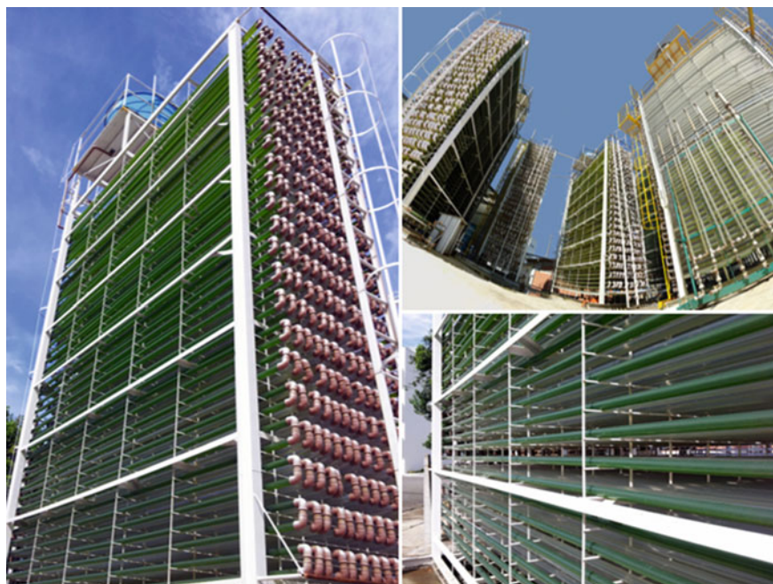
Fig. 17.2 Large-scale compact tubular photobioreactors for microalgae cultivation at NPDEAS (Curitiba, Paraná, Brazil)
