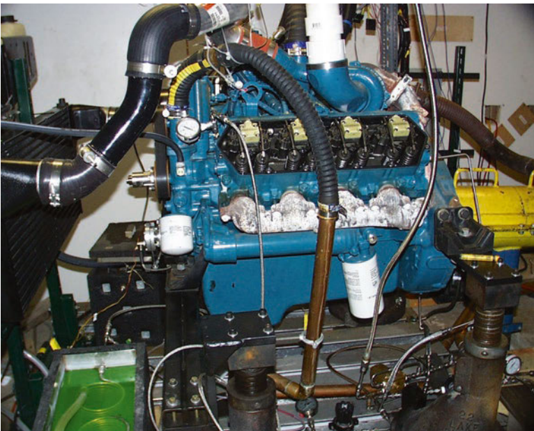
Fig. 4 Navistar T444E showing conversion to DME–diesel operation
