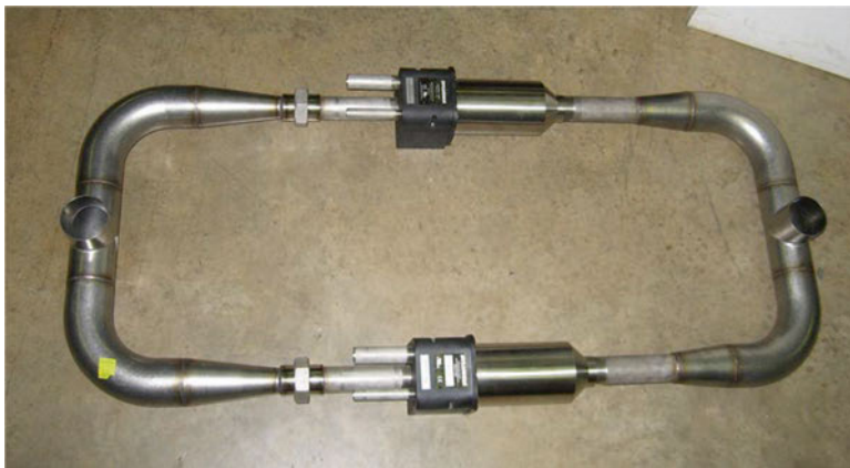
Fig. 6 Layout of the intake air heating system prior to installation on the engine stand [4]
