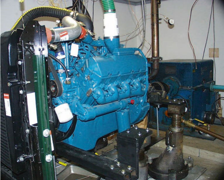
Fig. 3 Photo of the Navistar T444E Turbodiesel Engine in the 450 hp. engine test cell prior to conversion to DME–diesel blends
