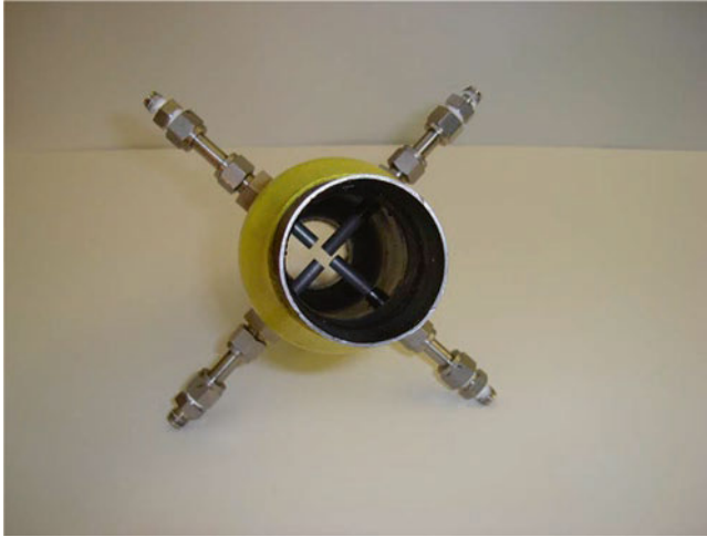
Fig. 5 Custom intake air manifold aspiration system used for fueling the engine, connected in front of an intake air heating system [4]
