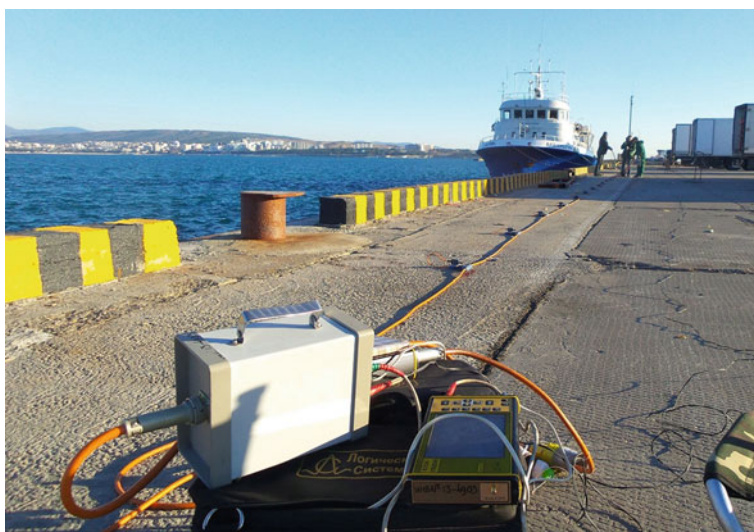
Fig. 2 Equipment for seismic prospecting (cable of geophones attached to the data storage device)
