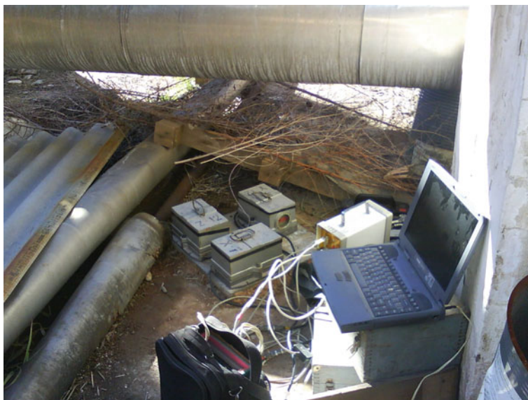
Fig. 1 Equipment for the 3-component PSM-PS ECWM survey (3-component seismic station)
