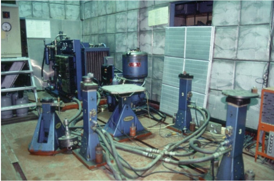
Fig. 3 Electrohydraulic shaking table “Fairy-22” (in the foreground) [23]
