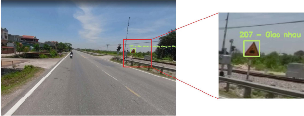
(c) Incorrect label detection cause small scale sign
