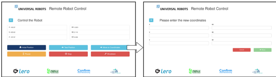
Fig. 2. The web application: The controller main page (left). Clicking the ‘Move to Coordinates’ button leads to the coordinates input page (right)
