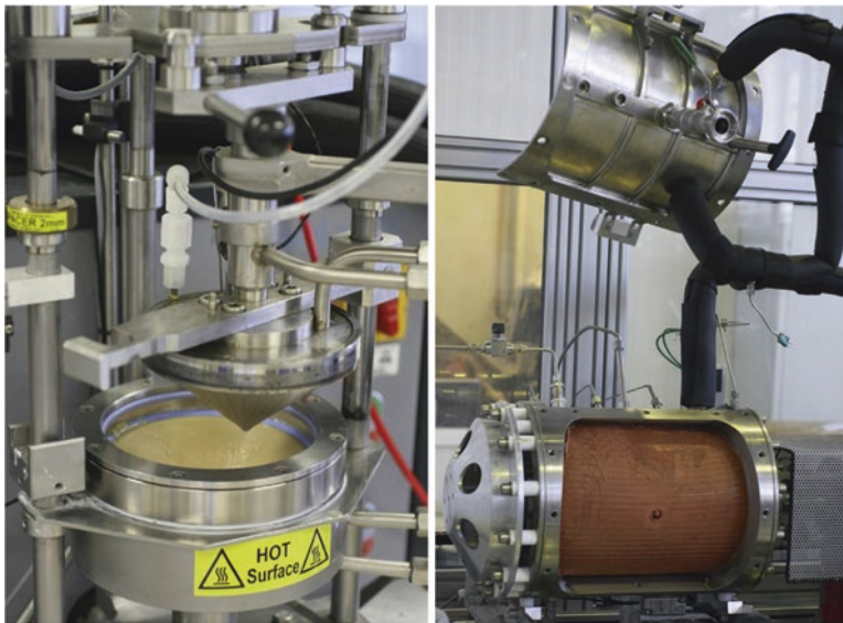
Fig. 6.6 Shear cell (left) and Couette cell (right) devices from the Laboratory of Food Process Engineering at Wageningen University (Kyriakopoulou et al. 2019)
