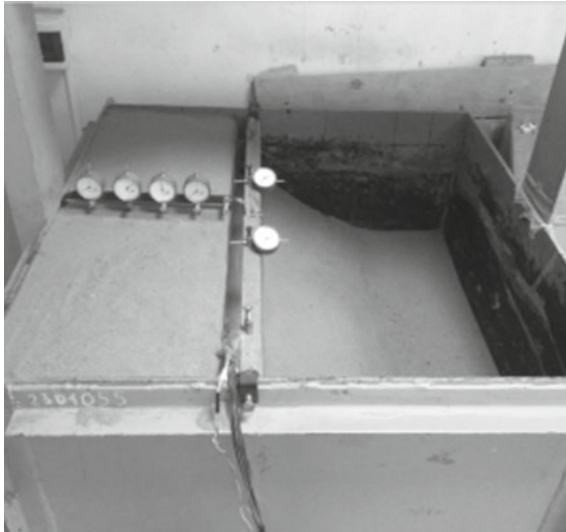
Fig. 2 Enclosing structure and counterweight soil berm mockup
