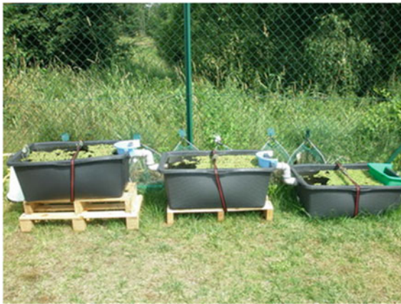
Fig. 2 Model of phyto- purification system using Azolla filiculoides
