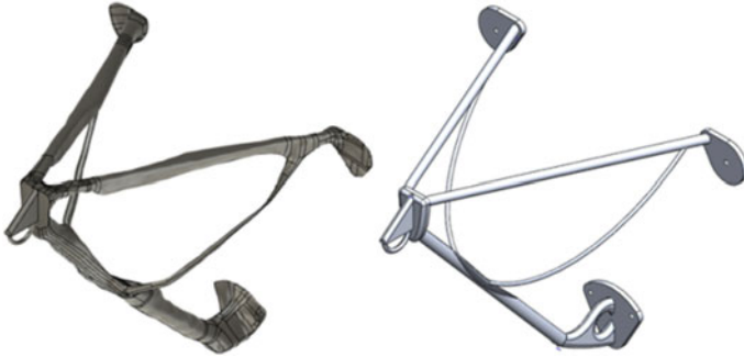
Fig. 3 Simplification of topology optimization results
