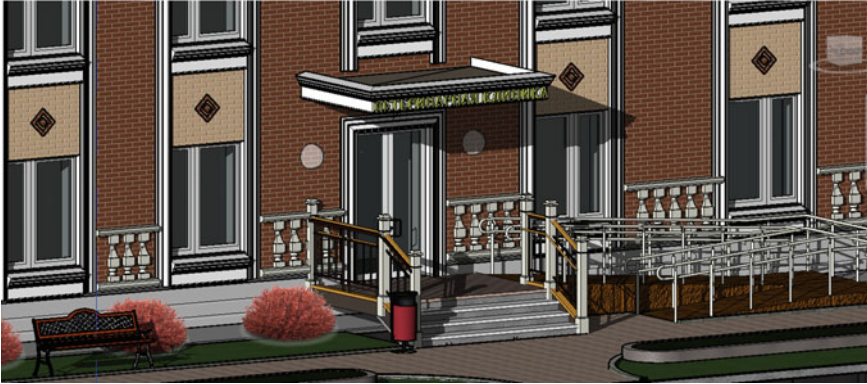
Fig. 4 Graphical representation of the LOD 500, the facade of the building with the surrounding area
