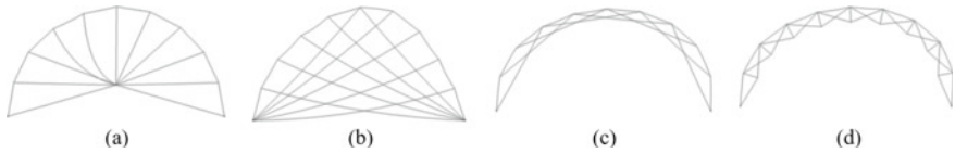
Fig. 4 Deformed schemes. a Arch № 1. Hud type system; b Arch № 2. Radial type system; c Arch № 3. Chord type system; d Arch № 4. Truss type system
