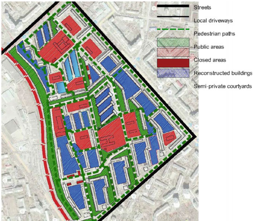
Fig. 4 Proposal for the organization of courtyards and public areas between Sovetskaya and Uralskaya streets
