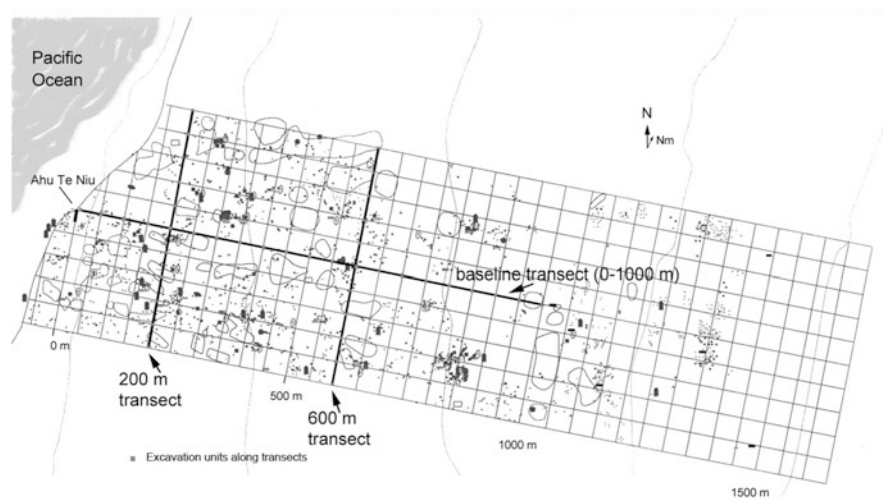
Fig. 18.2 Te Niu Survey Sector was a 500 m × 1600 m area divided into 50 m square units for the archeological survey and geomorphological study. Forty excavation units (50 cm × 50 cm) were placed every 50 meters along three transects, the prime East-West baseline, which extended from Ahu Te Niu to 1000 m up the western slopes of Maunga Terevaka, and two North-South transects perpendicular to the baseline transect at 200 m and 600 m from the ahu. Figure also illustrates the extent of household sites and gardens. Excavation unit location marked as small gray squares
