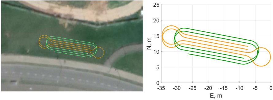
Fig. 1. Left: optimal field coverage for the particular working site. Right: target paths with constrained curvature for two robots operating simultaneously.
