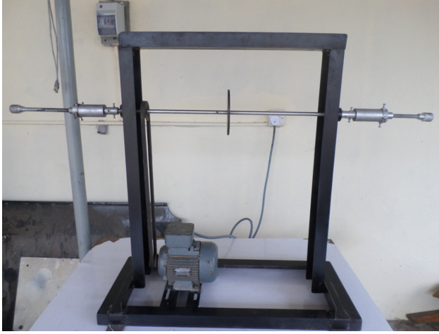
Fig. 3. The Piezoexciter Test Rig with the two exciters at both ends of the shaft.
