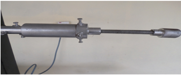
Fig. 4. Close up of the exciter assembly
