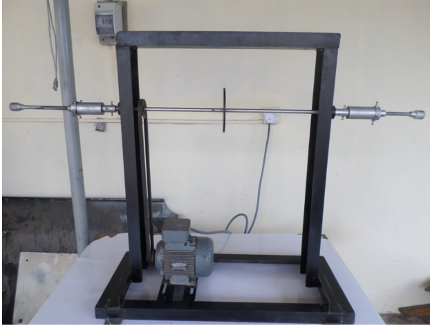
Fig. 3. The Piezoexciter Test Rig with the two exciters at both ends of the shaft.
