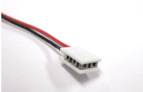
Fig. 9. Peltier element (TES1-1102LT125) [10]
