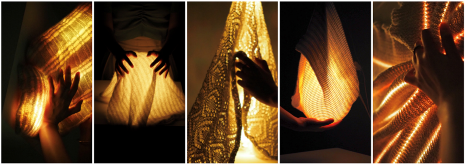
Fig.14. In the device interaction design, the interaction actions related to fabric materials are stretching, touching, repeatedly touching and stamping. The sensing methods are resistance change sensing and capacitance sensing. The feedback form is the increase of light intensity and the change of color temperature.
