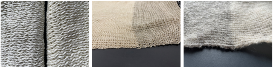
Fig. 11. Comparison of fabrics before and after mixed weaving of conductive yarn and non-conductive yarn.
