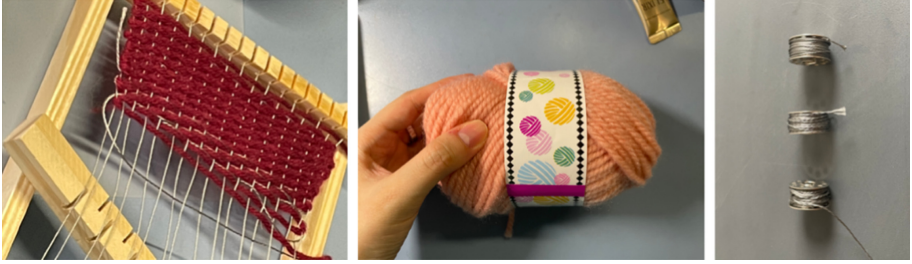
Fig. 9. Experiment D: mixed weaving experiment of wool and stainless-steel yarn. The woven method has higher requirements on the machine, and the conductive yarn with strong rigidity and low tensile property has poor tensile property.
