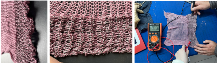
Fig. 6. Experiment A: mixed knitting experiment of cotton yarn and stainless-steel yarn. Because the stainless-steel yarn is made of strong strands, when the non-conductive yarn and stainless-steel yarn are mixed and woven, there will be obvious wrinkles, twisting and not sticking.
