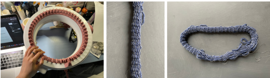
Fig. 8. Experiment C: mixed knitting experiment of wool and stainless-steel yarn. When knitting on a simple circular loom, the thread is often jammed and the machine often needs to be adjusted. In the textile process, it is very easy to twine and be off-line, which greatly increases the difficulty of mixed textile.
