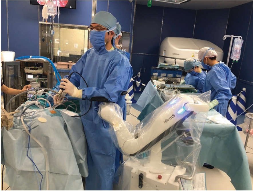
Fig. 5 This figure shows an intraoperative situation during endoscopic neurosurgery. The surgeon is standing beside one iArmS robot. The left hand, which holds the rigid endoscope, is supported by the iArmS. In intraoperative settings, a sterile drape covers the robot arm and the base of the iArmS. The arm holder is reused and sterilized independently to maintain sufficient friction between the surgeon's arm and arm holder
