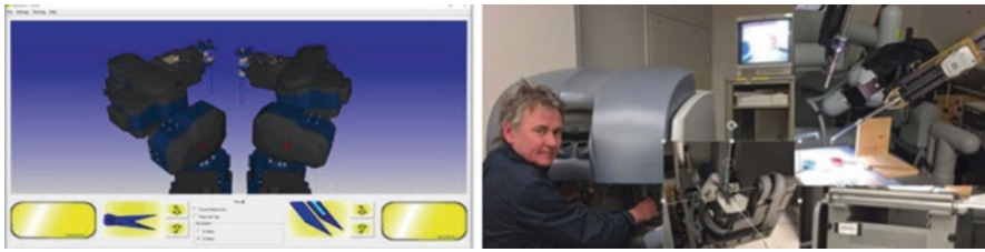
Fig. 2 Examples of VR simulators. On the left, an example of the Neuroarm simulator software; instruments can be selected and changed (here, scissors and scalpel). On the right, a picture of the 3D VR DaVinci simulator
