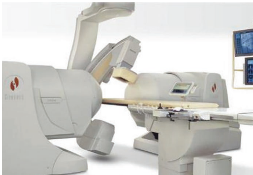
Fig. 5 Niobe by Stereotaxis. Figure source: Beasley RA. Medical robots: Current systems and research directions. J Robot. 2012;2012:1–14. (Obtained from “Open Access” sources under a CC-BY license)
