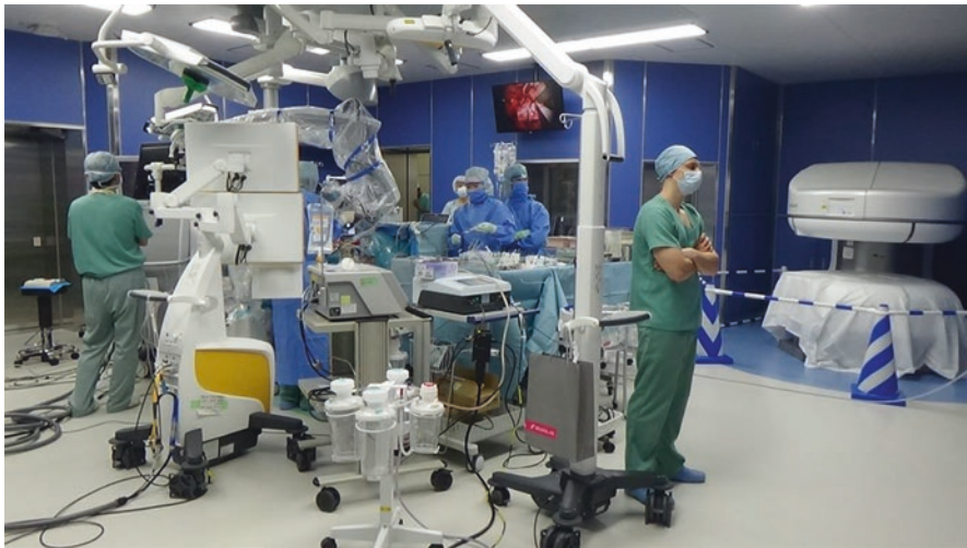
Fig. 1 The SCOT operation room; intraoperative MRI is installed in the same room. MRI, bipolar coagulator, a navigation system, and microscope are connected to the OPeLiNK through an Ethernet cable
