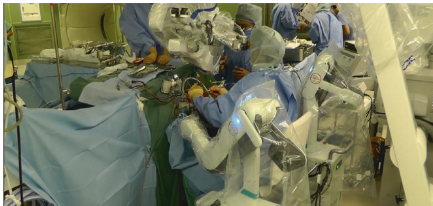
Fig. 4 This figure shows an intraoperative situation during microscopic neurosurgery. The surgeon sits on the surgical chair and two sets of iArmS robots are connected to it. Both arms of the surgeon are placed on the iArmS
