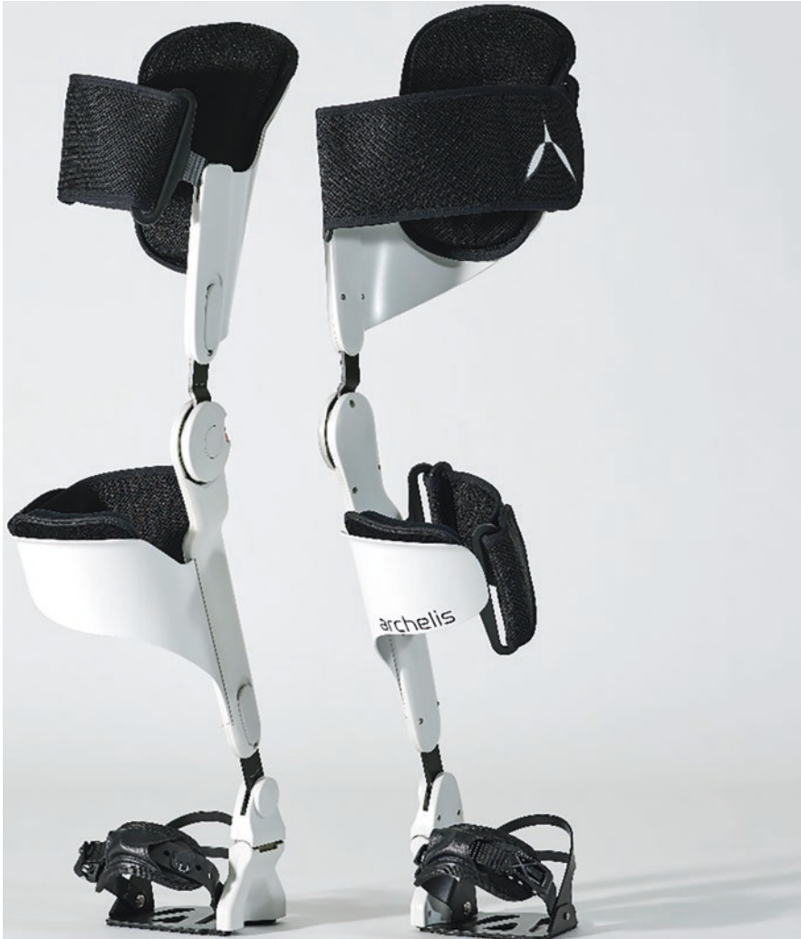
Fig. 6 This figure shows the left oblique view of the Archelis robot. The Archelis consists of two independent right and left parts. Its total weight is approximately 3.2 kg per extremity. The whitish hard part is fastened with Velcro to the surgeon's leg and lower back. (Image used with permission from Archelis Inc.)
