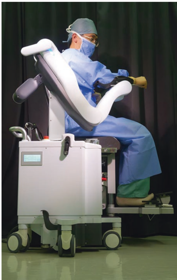
Fig. 2 This figure shows the iArmS robot with the surgeon in a sitting position. The iArmS is connected to the surgical chair and moves with it
