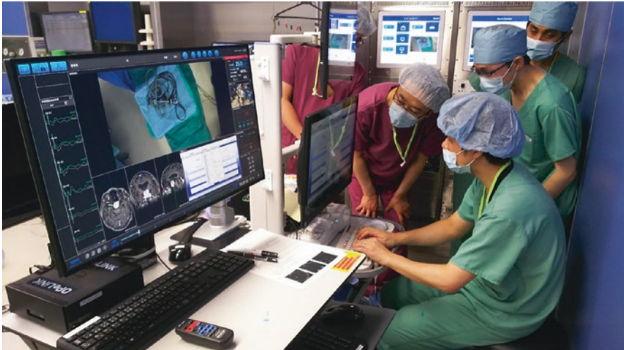
Fig. 5 Control desk of the wall monitor for OPeLinK on the left side of the picture, electrophysiological monitoring system on the right
