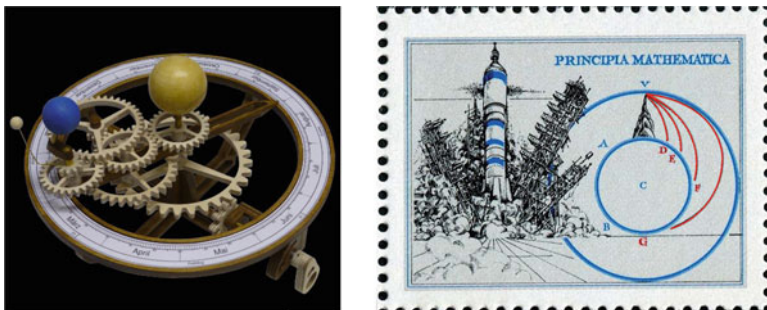
Fig. 6 Blasius [183] mechanism based on Hipparchus of Nicaea (190–120 BC) or Claudius Ptolemaeus (100–170 AD) deferent plus epicycles astronomical models; Newton's [105] diagram of cannonball sub-orbital and orbital trajectories
