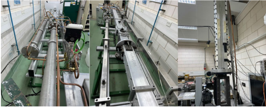
Fig. 8 Photo showing 3 out of 6 different shock tubes in the shock tube laboratory of the Dept. Mech. Eng., Ben Gurion University
