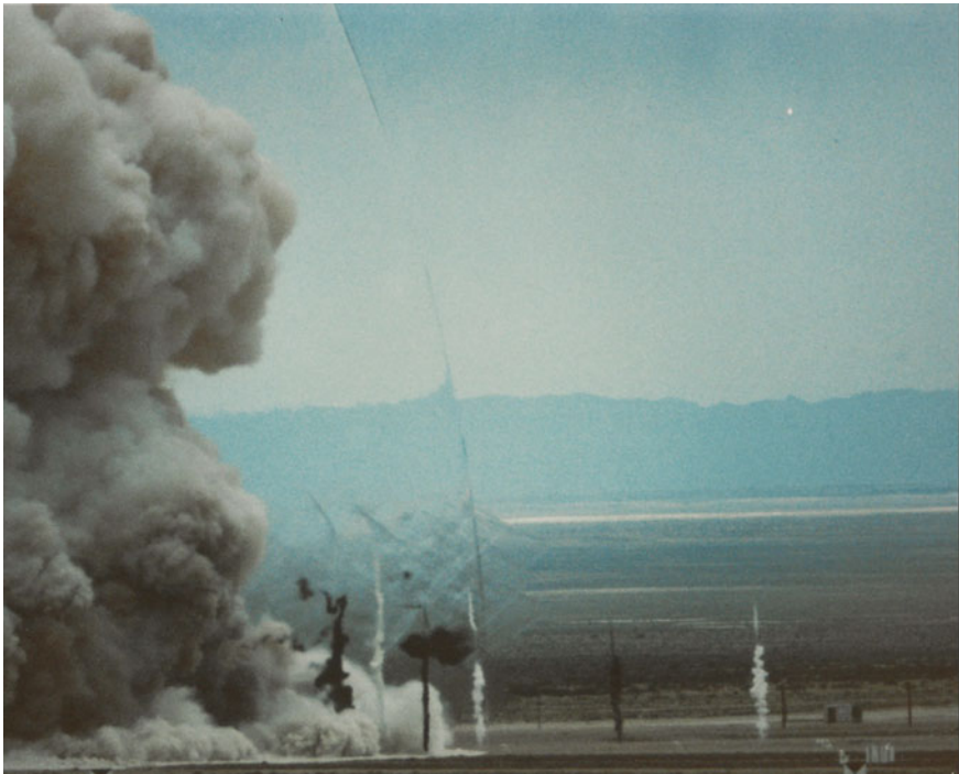
Fig. 9 The refractive image of the primary shock and the smoke tracers used to analyse the blast wave from a 2.218 Mkg surface burst ANFO explosion (MISERS GOLD)
