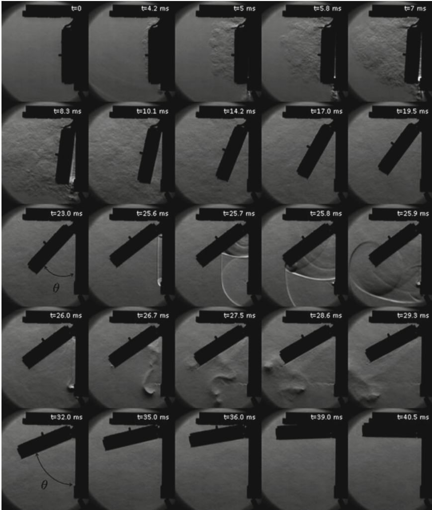
Fig. 20 Sequence of schlieren photos showing the impact of a normal shock wave ( M_{is} = 1.1 ), moving initially from right to left inside the shock tube, on an aluminum door. \theta is the angle between the door and its initial position
