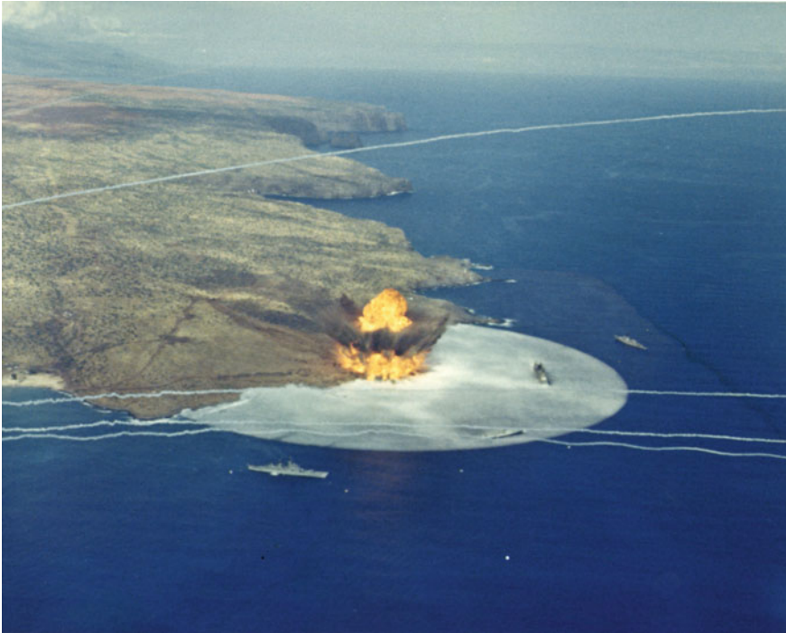
Fig. 6 SAILOR HAT, Shot No. 2 as the blast wave has just enveloped HMCS Fraser. The line of black smoke puffs can be seen to the left of the fireball. The two vessels outside of the blast wave are observational platforms thought to be at safe distances, but were struck by lava ejecta seen as the dark corona around the fireball
