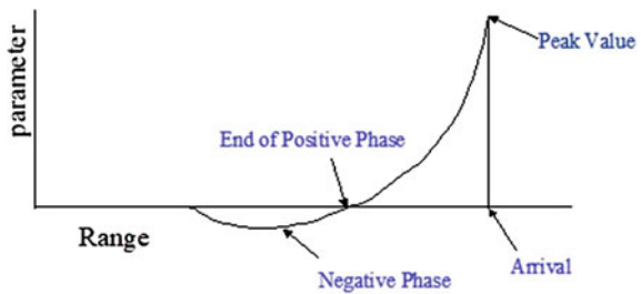
Fig. 8 Cartoon of a blast wave parameter as a function of range at a fixed time
