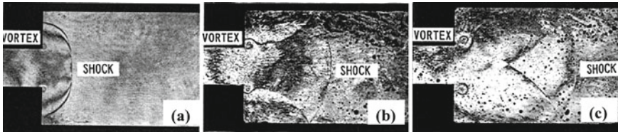
Fig. 8 Sequential interferograms. Weak shock generation from engine exhaust gas
