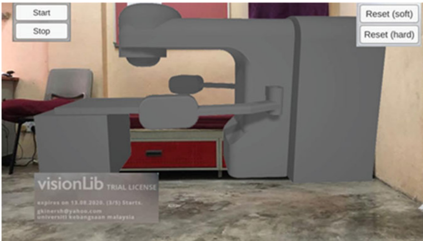
Fig. 6 Result of tracking an actual single size mattress with the LINAC model superimposed
