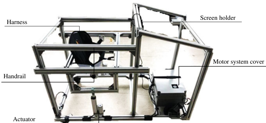
Fig. 2 The structure of PhyWalk product
