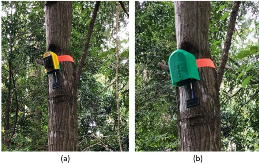
Fig. 2 The sensor modules that were installed on Mangifera foetida (Anacardiaceae); a sensor without weatherproof casing b sensor with weatherproof casing
