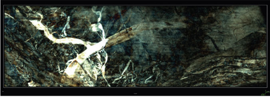
Fig. 11 RGB blend of three spectral decomposition volumes showing a time-slice through a fluvial channel complex. Subtle details become apparent compared to Fig. 3b which shows the same channel system using signal strength attribute
