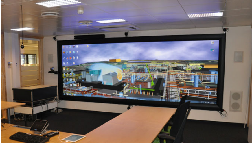
Fig. 1 Immersive display environment consisting of a back projected screen with infrared tracking cameras around the screen level
