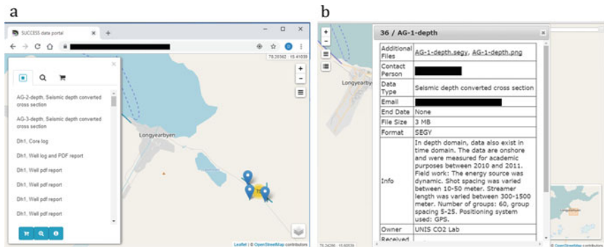
Fig. 10 a A scrollable list of all data visible on the map is shown in the left pane allowing the user to either select a dataset from the textual list or from the map. b When clicking on a dataset on the map or in the list, more information about the data shows up such as owner of data, email, data size, a short description, and a list of files associated with the data such as documents and measurements
