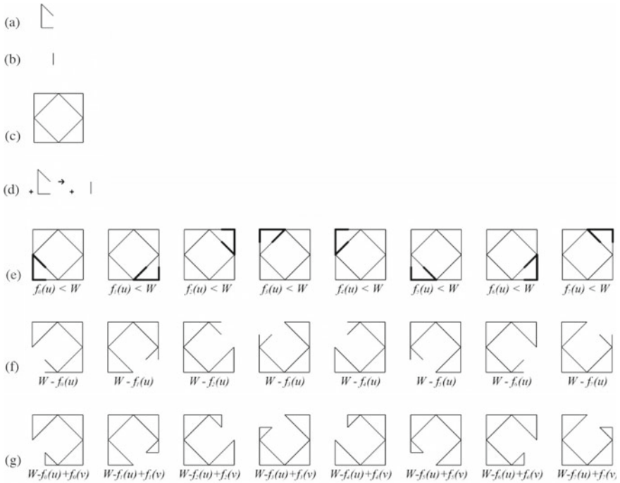
Fig. 1 A shape computation. a–c Shapes u , v , and W ; d Shape rule u \rightarrow v ; e Eight matches of the shape f(u) in W ; f Subtractions of the eight instances of the shape f(u) from W ; g Additions of the eight instances of the shape f(v) to the corresponding eight instances of the shape W - f(u)
