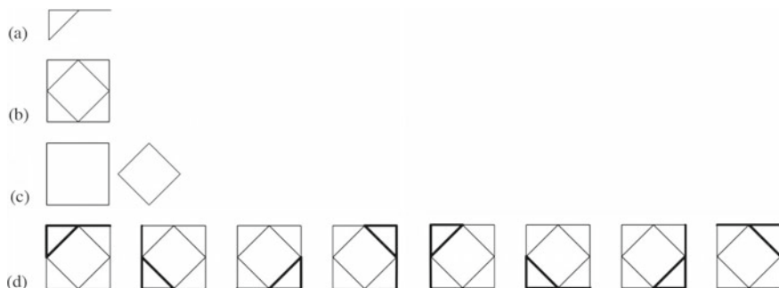
Fig. 3 An example of a restricted embedding of a subshape f(u) . All boundary points of the shape f(u) are registration points in the shape W . a Shape u ; b Shape W ; c Registered objects; d Eight transformations f embedding the shapes f(u) in W
