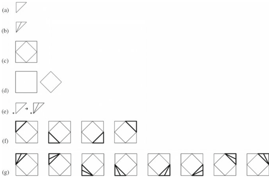
Fig. 6 An example of a calculation of counting non-equivalent embeddings and replacements of a shape f(u) shape by the shape f(v) . a Shape u ; b Shape v ; c Shape W ; d Registered objects; e Shape rule u \rightarrow v ; f Four embeddings of the LHS in W ; g Eight embeddings of the RHS in W
