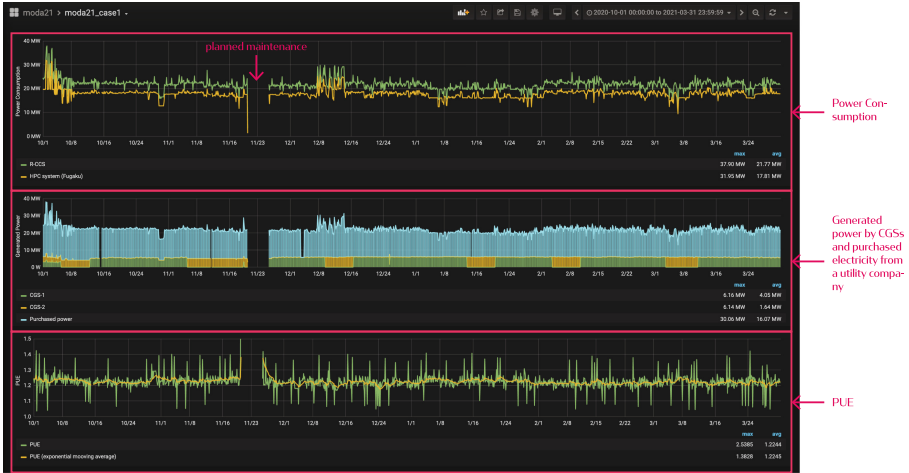
Fig. 2. A screenshot of electricity supply-and-demand and PUE during the prelaunch service period. The topmost graph (upper red box) shows power consumption for R-CCS as a whole and for the HPC system (only Fugaku). The middle graph (middle red box) shows the power generated by two CGSs and the purchased power from a public utility company. The bottommost graph (lower red box) shows the PUE and the exponential moving average of the PUE.
