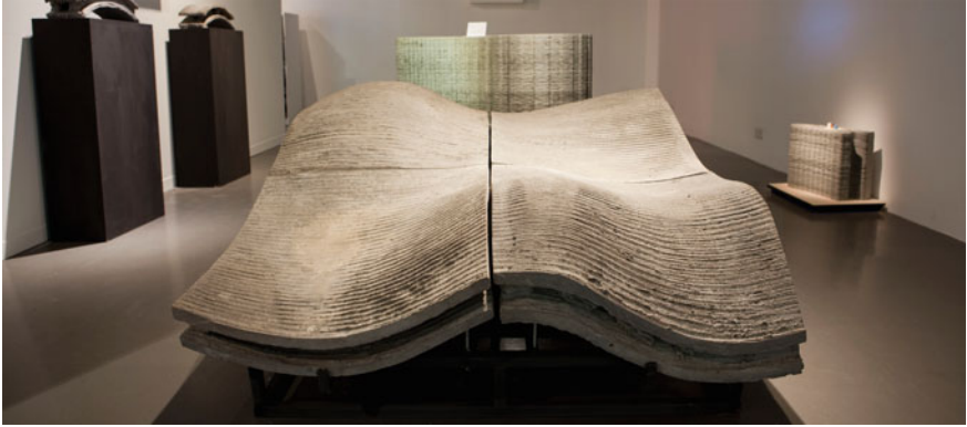
Fig. 2.7 Double-curved panels printed with conformal voids
