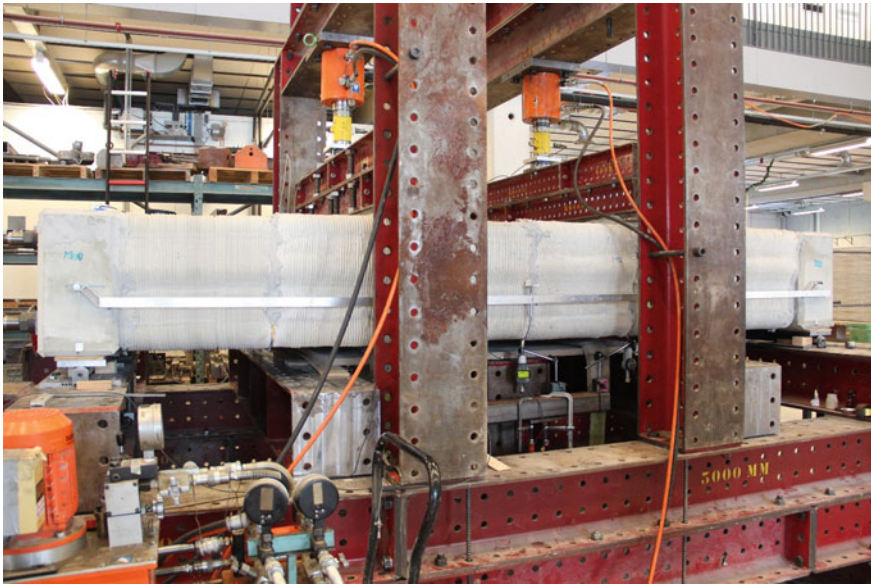
Fig. 2.6 Scale model in 4-point bending test set-up
