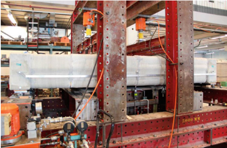
Fig. 6.13 Scale model in test 4-point bending test set-up (Theo et al. 2018)
