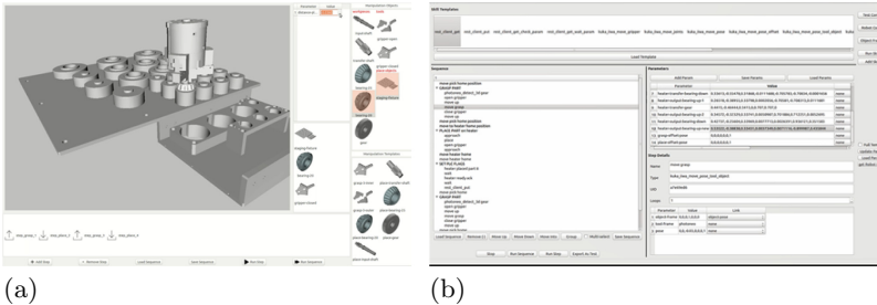
Fig. 4. (a) Modular programming GUI (b) Sequencing the skills through the GUI
