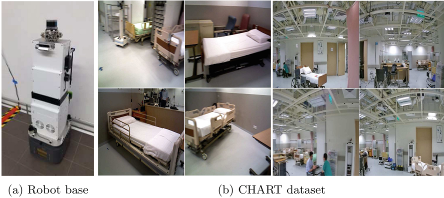
Fig. 1. (a) Our mobile robot base consisting of multiple visual sensors - six SONY IMX335 and two Structure Core cameras. (b) Our CHART dataset. The images collected in the hospital environment consist of multiple different hospital objects such as beds, tables, and wheelchairs. These images obtained from the visual sensors contain motion blur, occlusion, sensor noise, and significant distortion.
