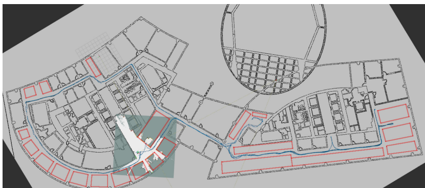
Fig. 7. The trajectory obtained with our localization approach (Blue) at level 9 floor in our office building. The white region is the PSLAM map dynamic frame. The red boxes are to show regions occluded with working cubicles in the real environment and it is not drawn in floor plan map in the experiment. (Color figure online)
