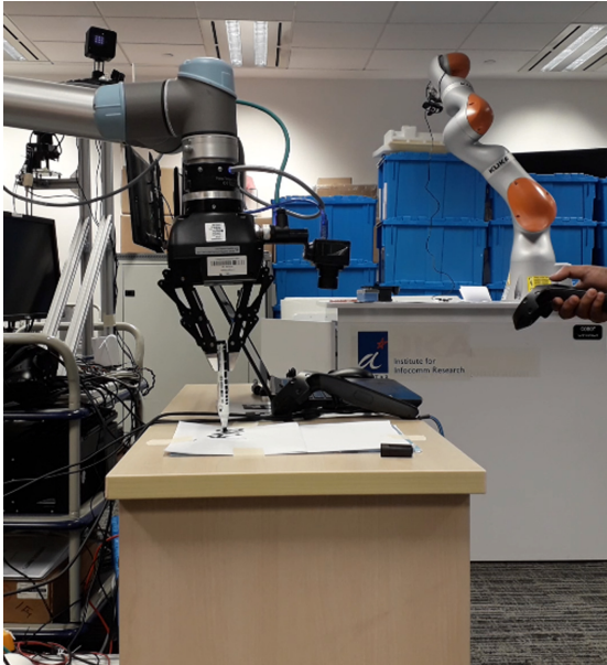
Fig. 2. Telemanipulation of UR5 Robot with HTC VIVE Controller.
