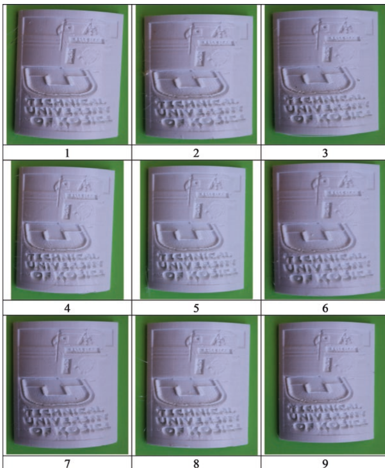
Fig. 15.22 Models of the different heights of the layer printed by the lithophane method
