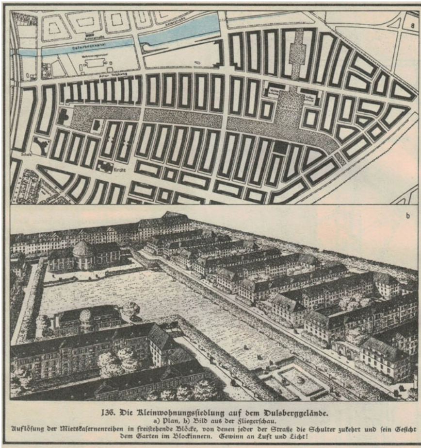
Fig. 7 Plan and perspective of Housing Estate Dulsberg with integrated green spaces and gardens inside the blocks. Source Wölflé, Karl, Hamburger Geschichtsatlas , Hamburg 1926, L. Friedrichsen and Co., p. 46
