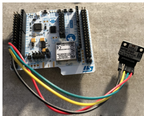
Fig. 4. ST P-Nucleo-WB55 and Bosch BME280 temperature sensor.
