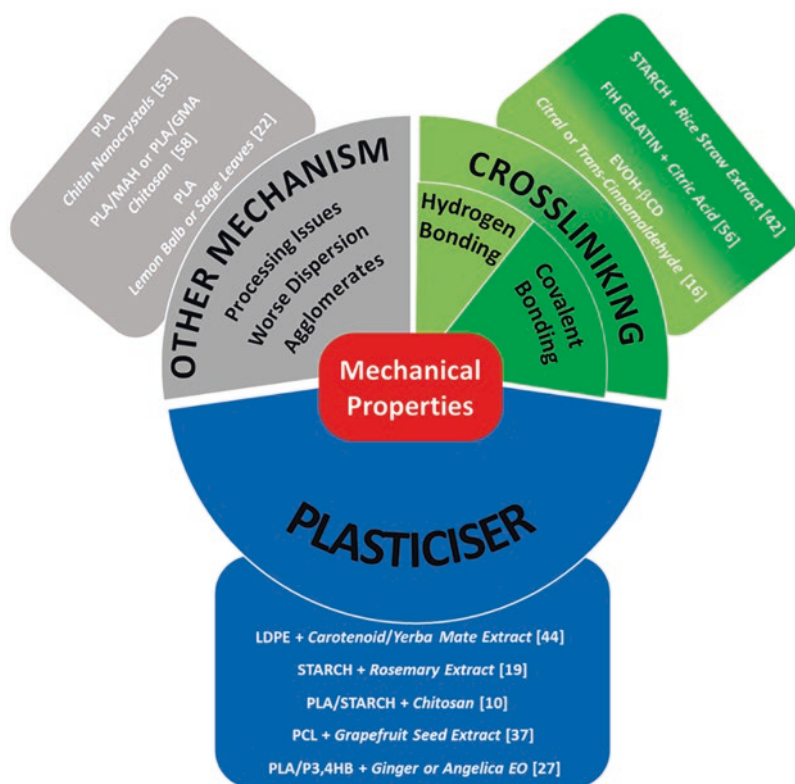
Fig. 8.6 Schematic representation of the various bioactive packaging films obtained by melt mixing/extrusion technique reviewed in this paragraph. They are catalogued according to the different interaction mechanisms among the bioactive compounds and the polymeric matrices, which are involved in the modification of mechanical properties of the resulting biocomposites
