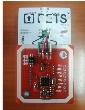
Fig. 5. NFC reader card connected to PETS Robot sub-board (i-COMEL)
