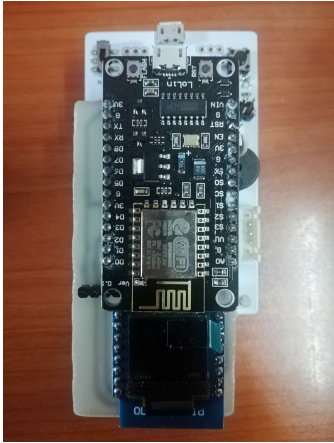
Fig. 6. ESP8266 board added to PETS Robot sub-board (i-COMEL)
