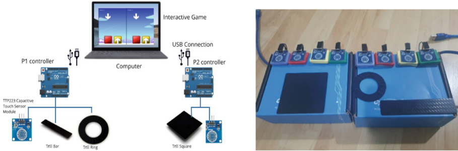
Fig. 1. General layout of the interactive tangible system (left), P2 and P1 controller (right)
