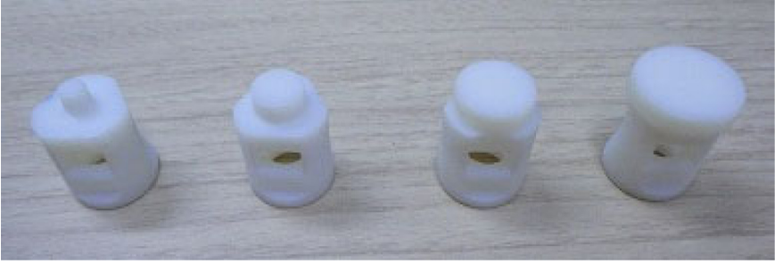
Fig. 4. Contact heads with different radii used in the experiment (from left to right: \varphi 5 , \varphi 10 , \varphi 15 , and \varphi 20 mm).
