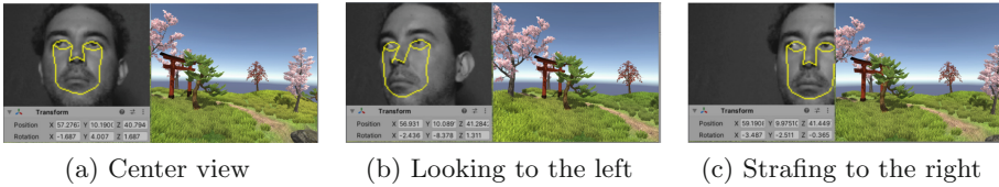
Fig. 1. Web camera head tracking controlling a virtual camera to increase immersion in non-immersive VR.
