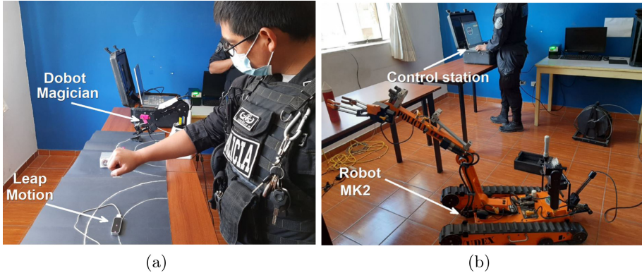
Fig. 3. Field tests. (a) With the DL01 interface. (b) With the MK2 robot keyboard interface.
