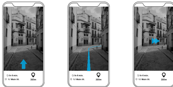
Fig. 1. AR information elements to navigate to the pick-up location (in blue). From left to right: orientation, path, node. (Color figure online)
