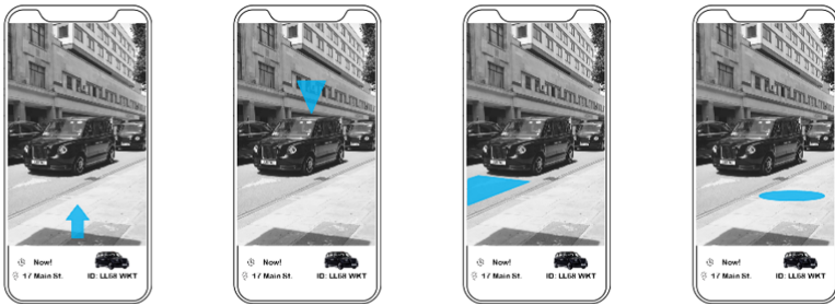
Fig. 3. AR information elements to identify the SAV (in blue). From left to right: orientation, vehicle highlighter, vehicle stopping area, customer boarding area. (Color figure online)
