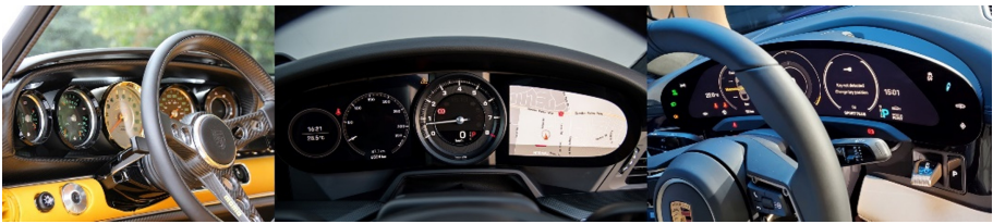
Fig. 2. From the classic instrument panel of 911 to the semi-digital instrument of the 992, to the new digital instrument cluster of Taycan.
