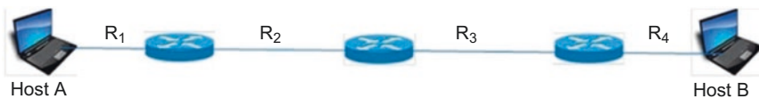
Fig. 2.9 Throughput for a file transfer from host A to host B with a single route
