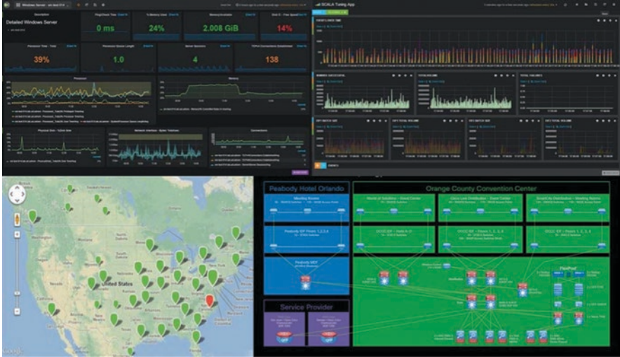
Fig. 1.4 Example of monitoring systems in a network operations center
