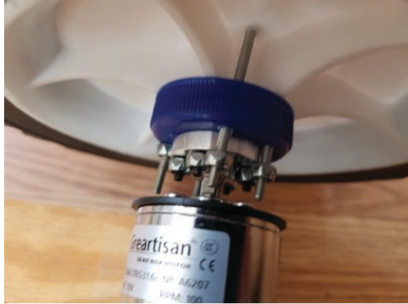
Fig. F.6 Wheel mounted onto DC motor
