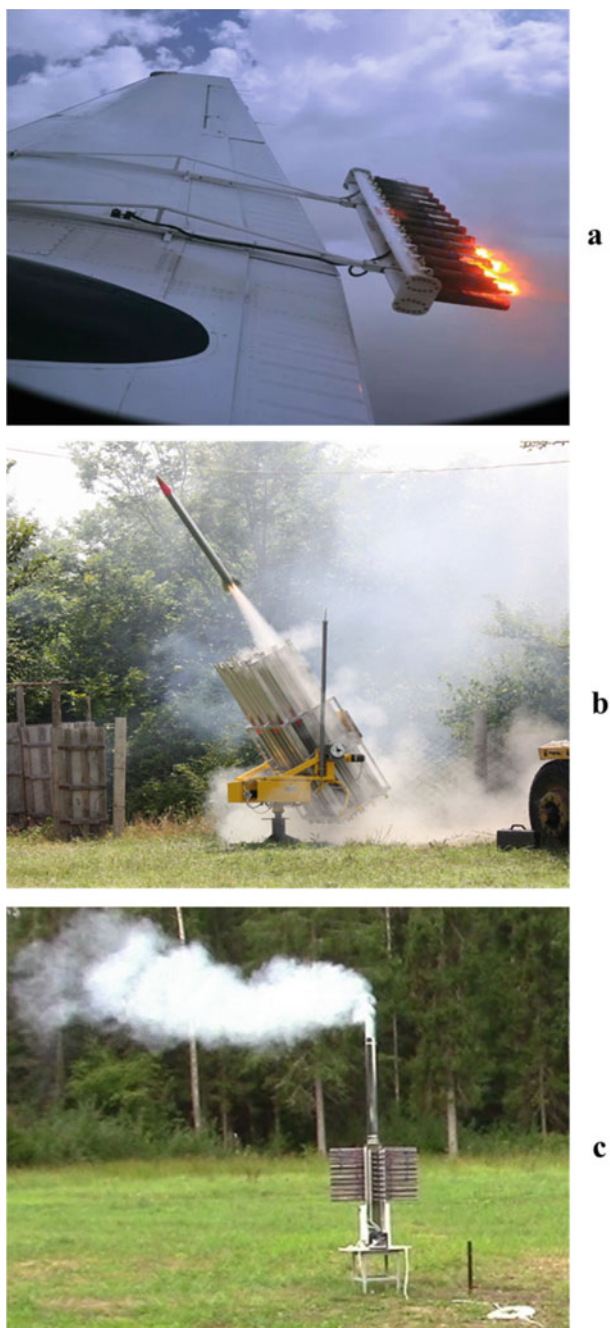
Fig. 2.3 Technical systems for delivering seeding materials into clouds and their environments: a airborne pyroflares; b small-sized anti-hail rocket “Alazan-6” and automated anti-hail launcher “ELIA-2”; c liquid acetone-based ground generator. Sources a National Center of Meteorology of the United Arab Emirates; b Magomet Abshaev; c Viktor Korneev; all used with permission
