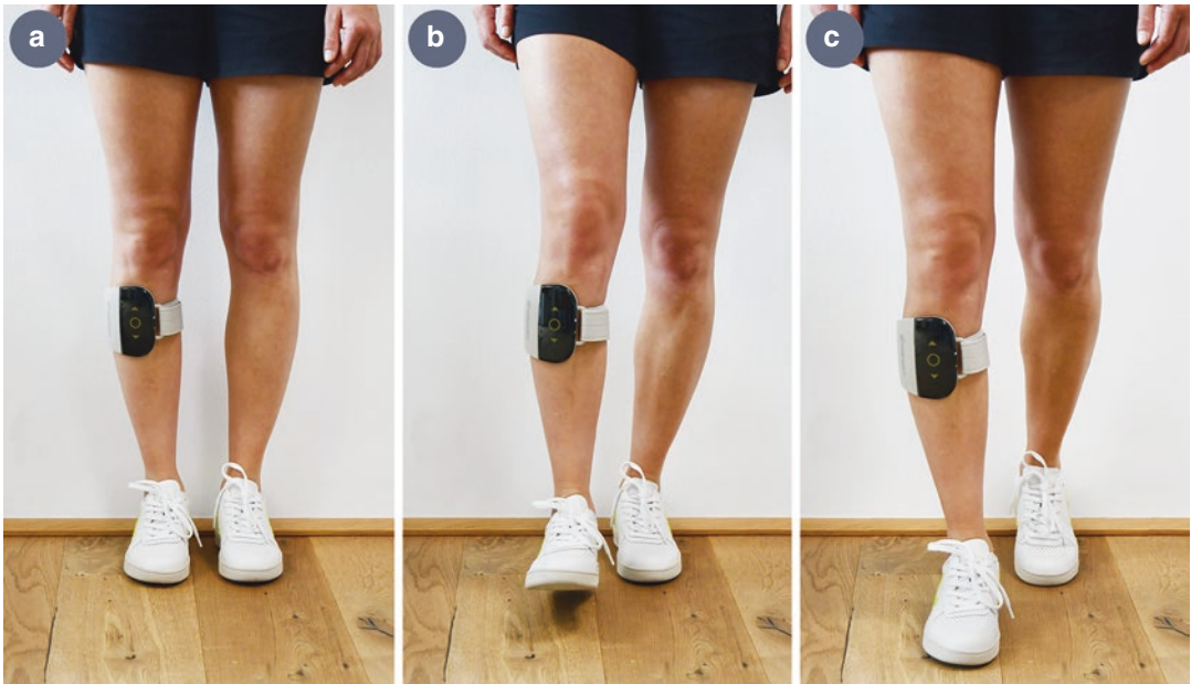
Fig. 7.2 A myoelectric orthosis stimulates the peroneal nerve to lift the foot during the swing phase, utilizing a tilt sensor and accelerometer technology; shown in the stance
