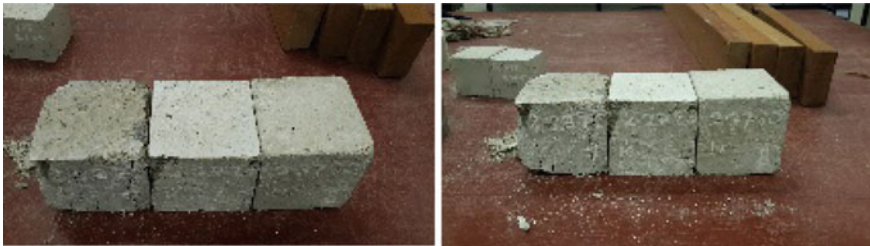
Fig. 22.8 Failure mode of the specimen with 1.00% of TiO 2
