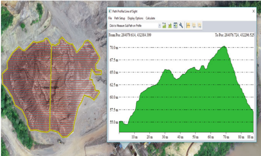
Fig. 5.11 Vertical cross section of stockpile
