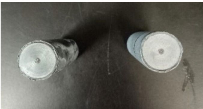
Fig. 19.11 Typical fractures on surfaces of specimen after tensile test
