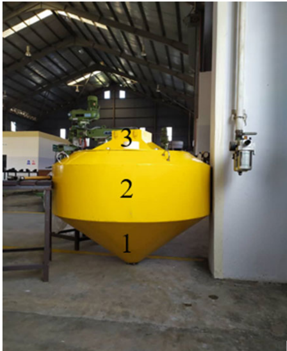
Fig. 33.7 Complete installation of modular buoy
