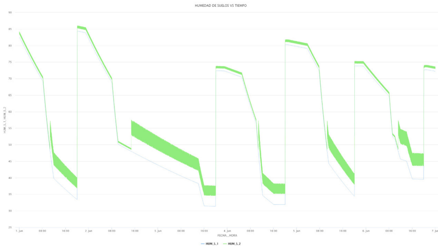
Fig. 29. Graph of soil moisture vs. time for automatic irrigation every twenty-four hours
