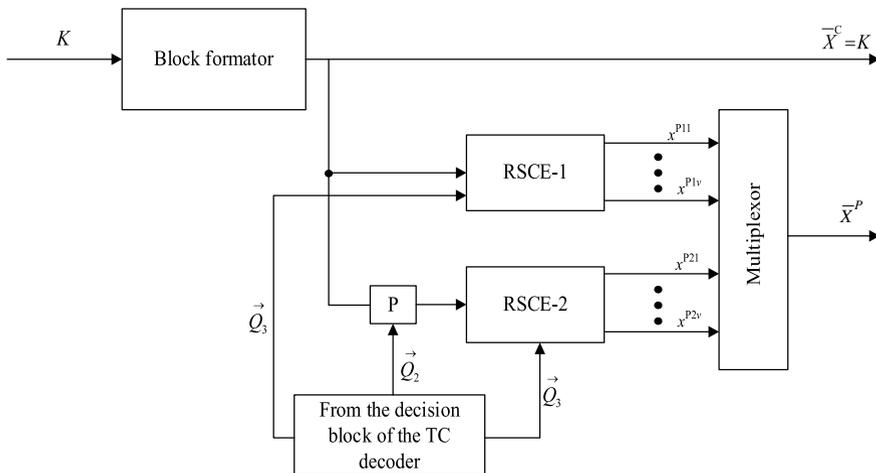
Fig. 1 Block diagram of the modified TC encoder
