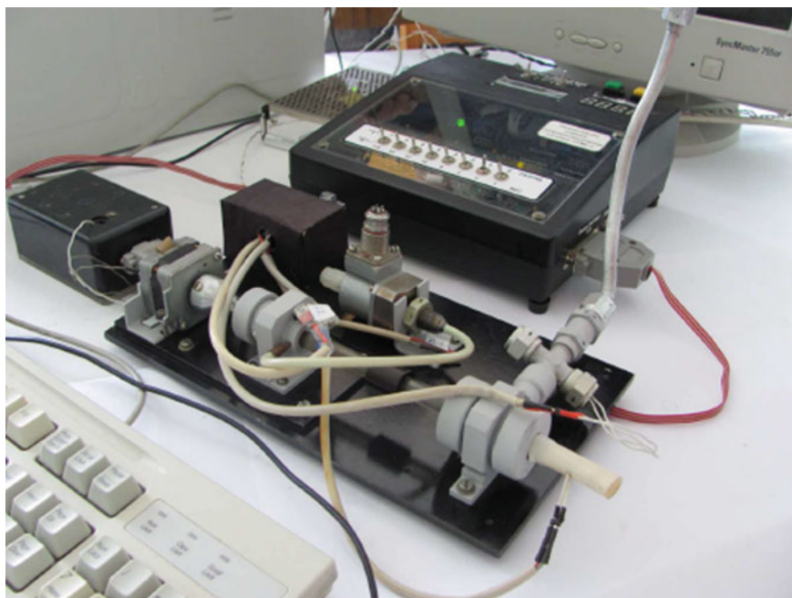
Fig. 1 The view of the experimental setup of vortex energy separator
