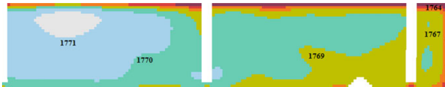
Fig. 8 Vertical cross-section of predicted heat field (in Kelvins) at the line of outlets ( y = 1.3 m) for comparison with data in [5]
