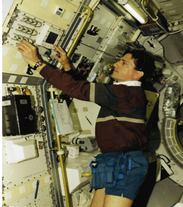
Fig. 4.2 NASA Astronaut D. Thomas operating TEMPUS on board the Space Shuttle Mission STS-83. (Photo: NASA)
