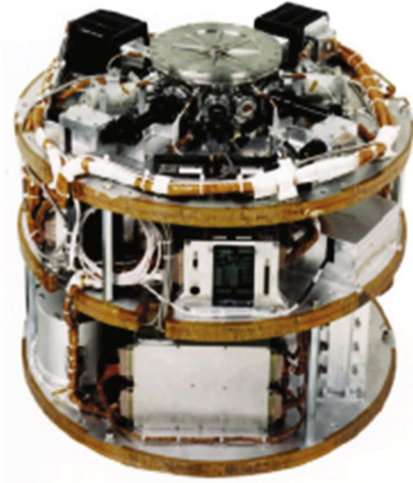
Fig. 5.3 Picture of an electrostatic levitation furnace flown in the sounding rocket TR-IA#7. Hardware design was similar to the one in Fig. 5.2, but the number of heating lasers was reduced to 2 due to size and power limitation
