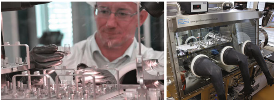
Fig. 3.11 Sample integration process using the EML glovebox
