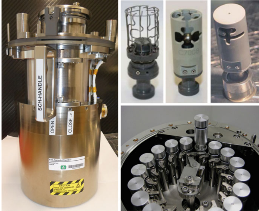
Fig. 3.7 (Left) EML sample chamber. (Top right) Three sample holder types: cage, cup and chill-cool-plate. (Bottom right) View inside sample chamber's vacuum part with sample carousel holding 18 dummy sample holders and the sample launch lock mechanism
