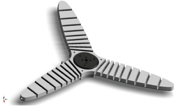
Fig. 1.7 Gripping jaw in final form
