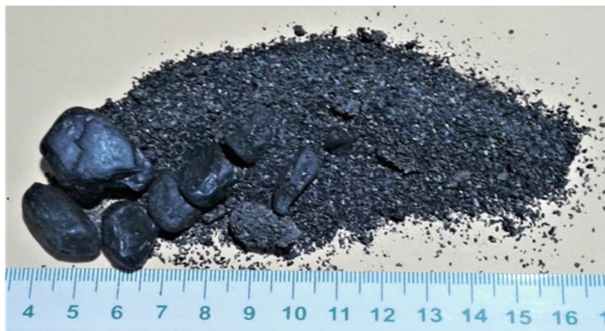
Fig. 12 Image of a typical bed sediment sample of the Gallegos River collected at a point bar. The mostly silt and sand grain-size sample includes large coal fragments (i.e. ~0.5–1.0 cm)
