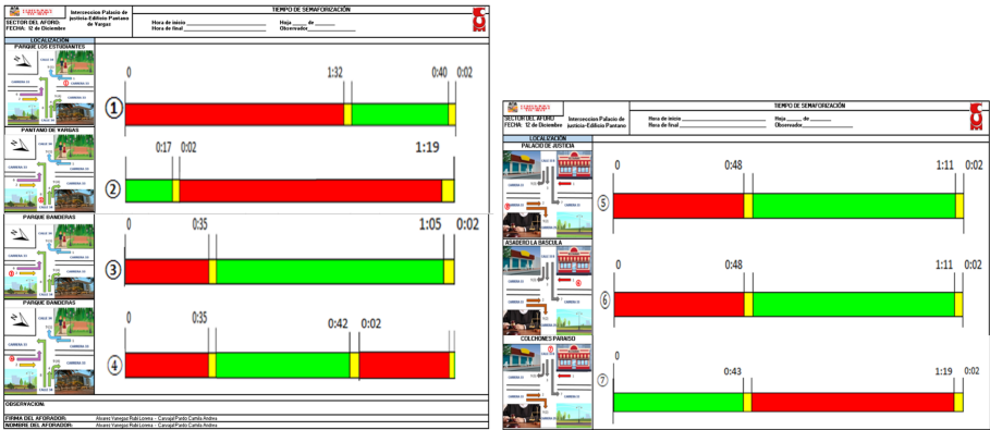
Fig. 6. Traffic lights phases for the intersections. Left, for intersection 1 and Right for intersection 2.
