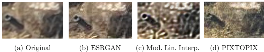
Fig. 5. Prediction of the implemented techniques, (a) Original Image, (b) ESRGAN Network, (c) Technique, (d) PIX2PIX Network
