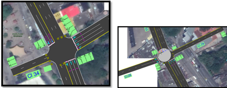
Fig. 9. Vehicle flows per lane and allowed turns of the current state. Left image, for intersection 1. Right image, for intersection 2.
